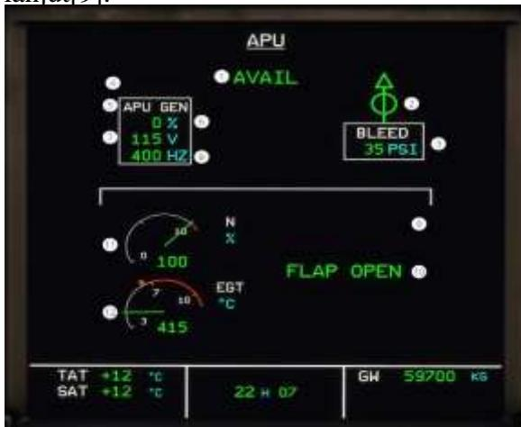
Gambar 5. APU EGT (Exhaust Gas Temperature)
