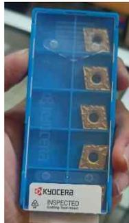
Gambar 6. Karbida Sisipan CNMG120404PS
