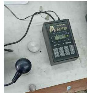
Gambar 8. *System Affri Portable Brinell Hardness Test*
