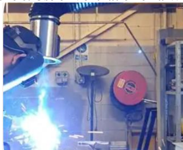
Figure 6. Use of Ventilation on a Welder
