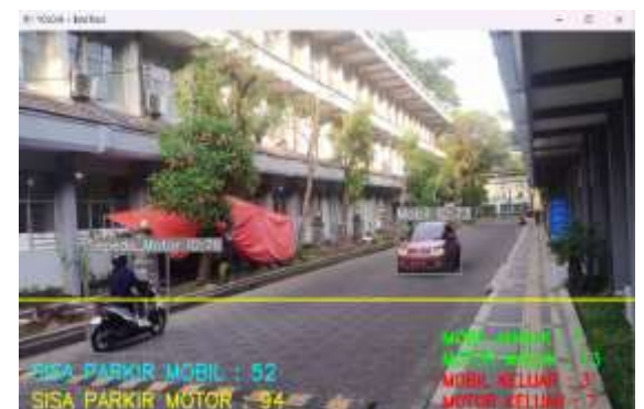
Figure 11. Car and Motorcycle Simultaneous Entry and Exit
