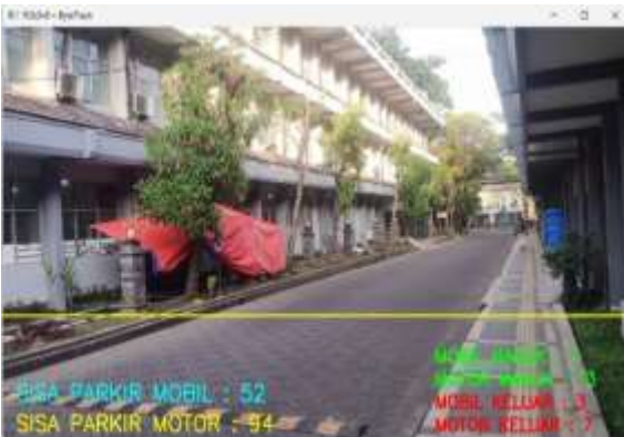
Figure 14. Vehicle Counting Accumulation Display
