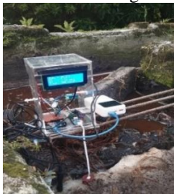
(a) Liquid waste storage tank 0 M (300 NTU)
