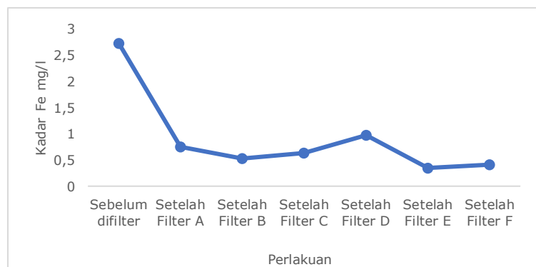
Figure 6. Kurva Variasi komposisi filter terhadap adsorpsi Fe
